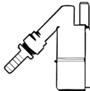
Rupture de charge (Air-Gap)
